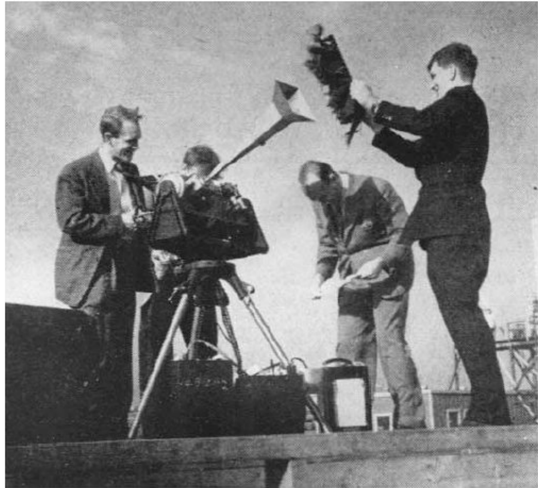
Fig. 1. Early 1.5 cm microwave radiometer atop a Radiation Laboratory building at M.I.T. Measurements are being made by (left to right) E. Beringer, R. Kyle, A. Vane, and R. H. Dicke. Dicke is shaking the “shaggy dog” — a piece of absorbing material used as a 295 K calibration source.
