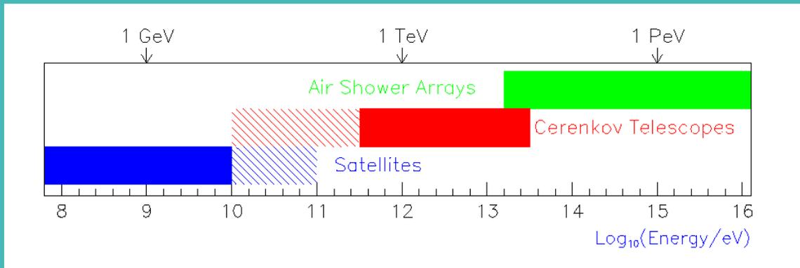
STACEE is sensitive to the range of gamma-ray energies between 50 and 500 GeV. This region of the electro-magnetic spectrum lies beyond that currently explored by satellite experiments and below the threshold of existing Imaging Cherenkov Telescopes.
