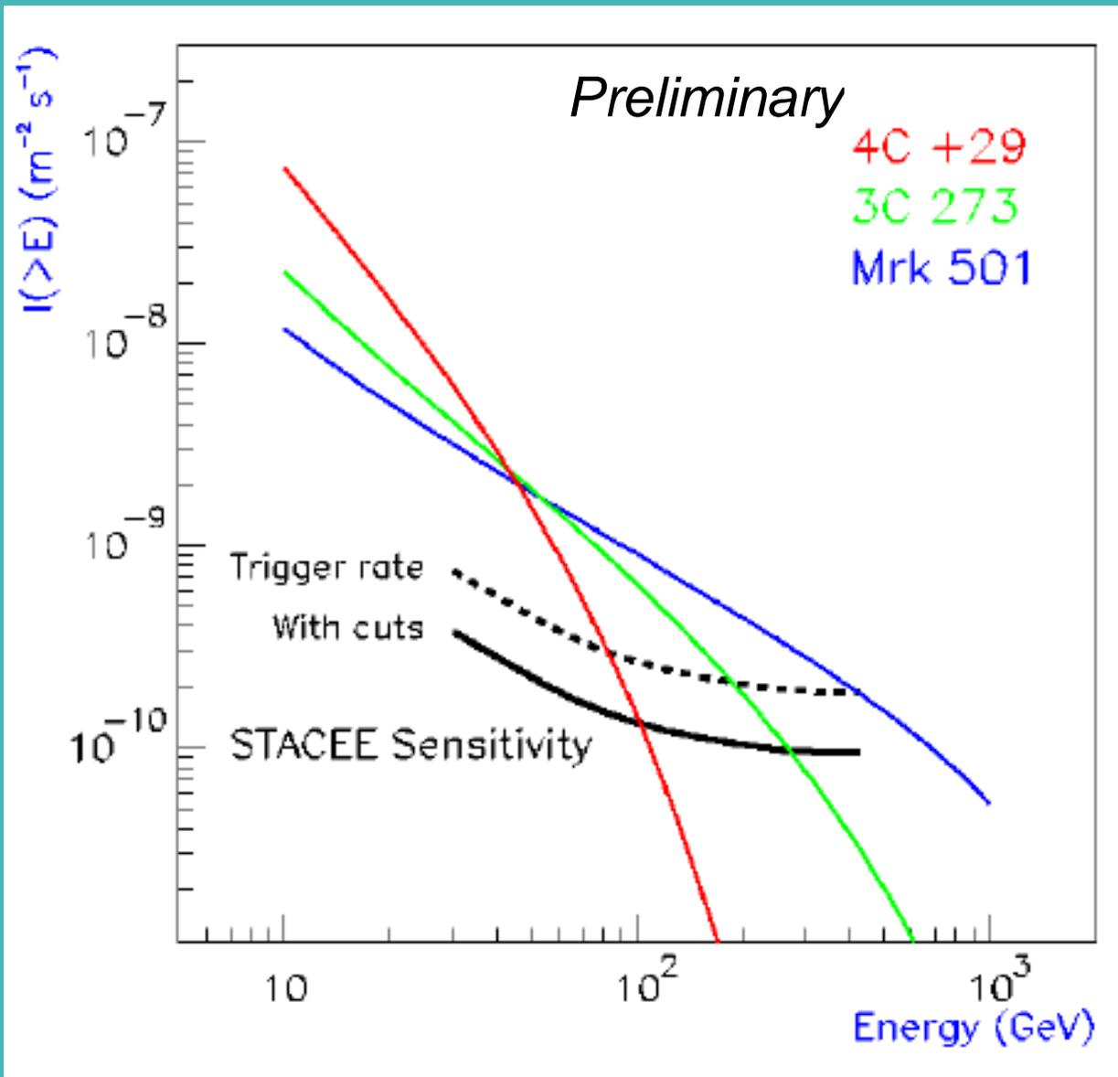
A sensitivity estimate for the completed STACEE experiment is shown above. Extrapolated EGRET spectra (with estimated extragalactic absorption) for sample sources are also shown.
