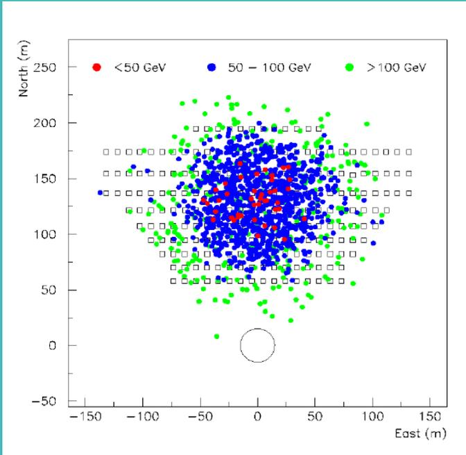
The triggering probability of simulated showers is used to calculate the effective collecting area of the array. Convolution of this area with an assumed source spectrum of  $E^{-2}$  yields an energy threshold of  $\sim 115$  GeV for a source at zenith
